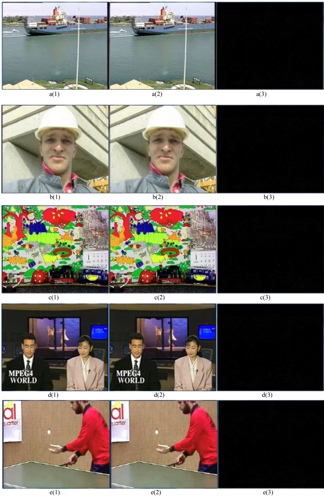
Fig. 2. Column 1 are unmarked H.264/AVC compressed/decompressed frames (QP=24 and 50 th frame), Column 2 are marked H.264/AVC compressed/decompressed frames, and Column 3 are the difference between the unmarked and marked decoded frame.
