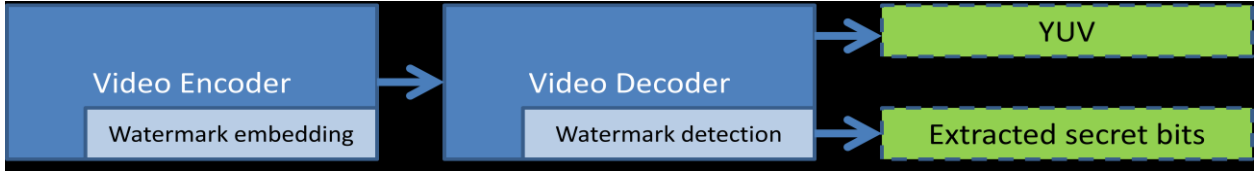
Fig.1. Embedding and detecting flowchart
