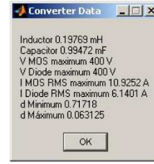
Fig. 4. Results on boost PFC converter.
