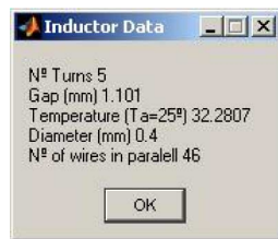
Fig. 11. Data for making the inductor.
