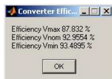
Fig. 7. Efficiency of the boost converter.
