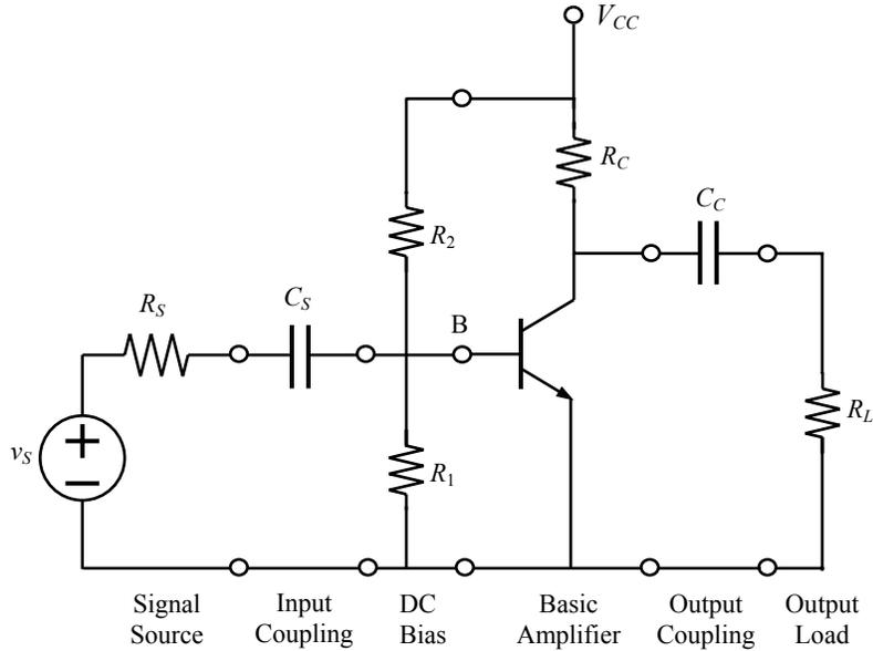
**Figure 1** A stage of an amplifier circuit.
