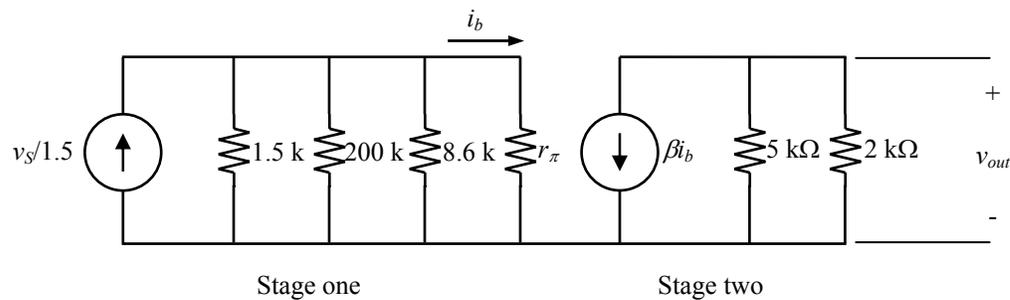
**Figure 3:** Small-signal circuit of the BJT amplifier.
