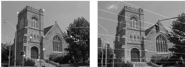
Figure 9: Epipolar geometry estimated from a filtered match set: the epipolar lines corresponding to selected points on the left image.
