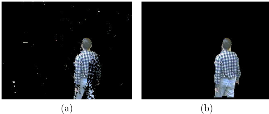
Figure 4.1: (a) an image of a person’s silhouette extracted without the use of either median filtering or morphological operations; (b) an image of a person’s silhouette extracted with the use of both median filtering and morphological operations
