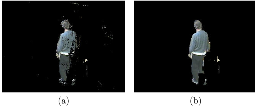
Figure 4.2: (a) an image of a person's silhouette extracted without the use of either median filtering or morphological operations; (b) an image of a person's silhouette extracted with the use of both median filtering and morphological operations
