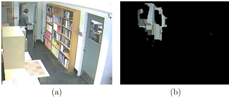
Figure 4.4: (a) an image of a person who is in between the camera and a recently opened door; (b) an image showing the result of segmentation
