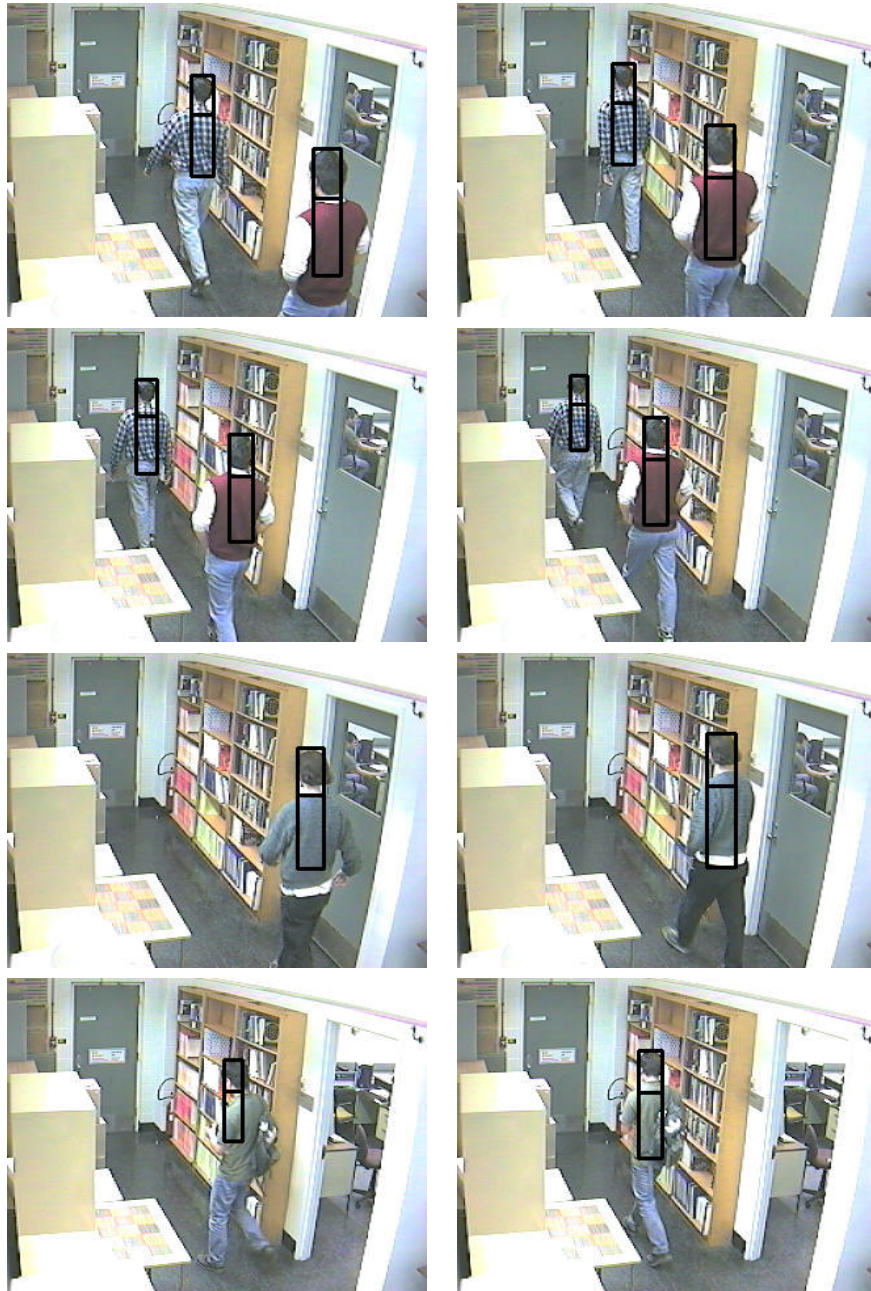
Figure 6.3: sample images showing 4 detected persons, their head regions and the colour extraction regions
