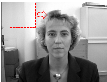
Figure 3.1.1: Sweeping window scans the image [68] from the top-left corner to the bottom-right corner to find a face
