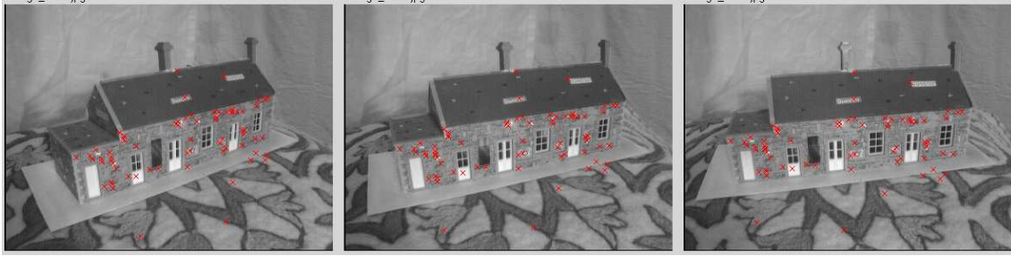
Figure 4.6: Correspondences in the support set for the trilinear tensor of the first 3 images.
