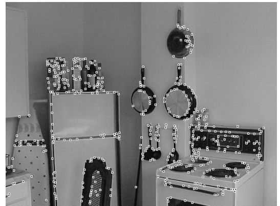
Figure 4: The corners extracted by the SUSAN corner detector, for the Kitchen image pair (approximately 500 per image).
